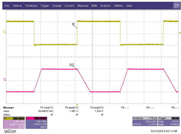
Figure 12. Inverting Large Signal Step Response
