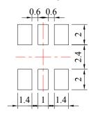
Unit: mm Tolerance: ± 0.10mm
