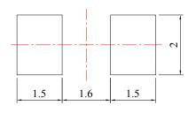
Unit: mm Tolerance: ± 0.10mm
