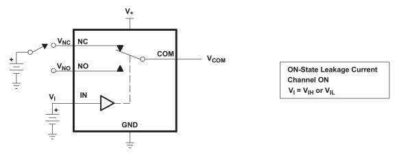
Figure 16. ON-State Leakage Current ( $I_{COM(ON)}$ ,  $I_{NC(ON)}$ ,  $I_{NO(ON)}$ )
