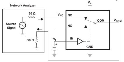
Channel ON: NC to COM  $V_I = V_+$  or GND
