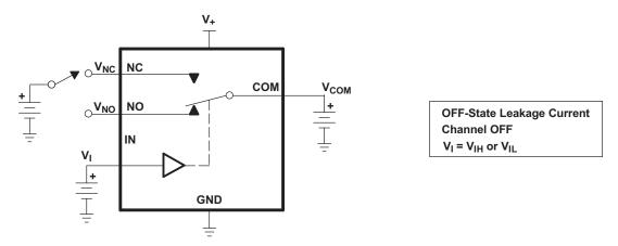
Figure 15. OFF-State Leakage Current (I<sub>NC(OFF)</sub>, I<sub>NC(PWROFF)</sub>, I<sub>NO(OFF)</sub>, I<sub>NO(PWROFF)</sub>, I<sub>COM(PWROFF)</sub>)
