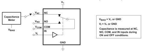
Figure 17. Capacitance (C<sub>I</sub>,  $C_{COM(ON)}$ ,  $C_{NC(OFF)}$ ,  $C_{NO(OFF)}$ ,  $C_{NC(ON)}$ ,  $C_{NO(ON)}$ )
