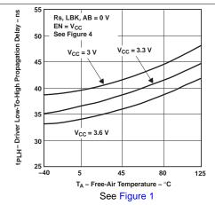
Figure 9. Driver Low-to-High Propagation Delay vs Free-Air Temperature
