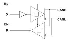
Figure 30. SN65HVD34 Functional Block Diagram
