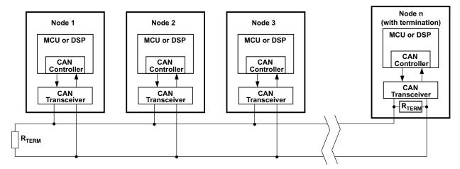
Figure 37. Typical CAN Bus
