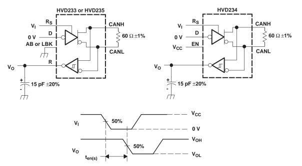
NOTE: All V<sub>1</sub> input pulses are supplied by a generator having the following characteristics: t<sub>r</sub> or t<sub>f</sub> ≤ 6 ns, pulse repetition rate (PRR) = 125 kHz, 50% duty cycle.
