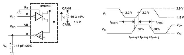
NOTE: All V<sub>1</sub> input pulses are supplied by a generator having the following characteristics:  $t_r$  or  $t_f \le 6$  ns, pulse repetition rate (PRR) = 125 kHz, 50% duty cycle.
