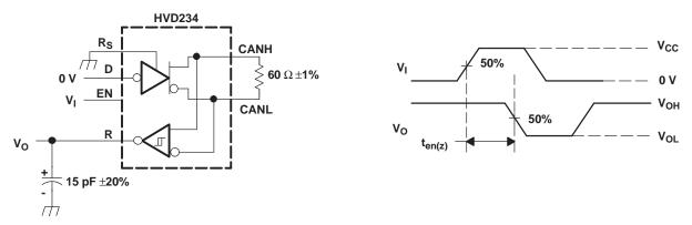
NOTE<sup>:</sup> All V<sub>I</sub> input pulses are supplied by a generator having the following characteristics:  $t_r \text{ or } t_f \leq 6 \text{ ns}$ , pulse repetition rate (PRR) = 50 kHz, 50% duty cycle.
