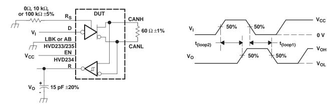
NOTE<sup>:</sup> All V<sub>I</sub> input pulses are supplied by a generator having the following characteristics:  $t_r$  or  $t_f \le 6$  ns, pulse repetition rate (PRR) = 125 kHz, 50% duty cycle.
