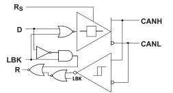
Figure 29. SN65HVD33 Functional Block Diagram
