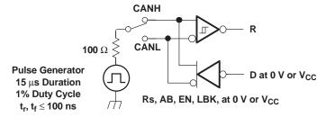
NOTE: This test is conducted to test survivability only. Data stability at the R output is not specified.
