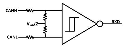
Figure 35. Simplified Recessive Common Mode Bias and Receiver
