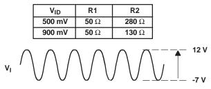
NOTE: All input pulses are supplied by a generator with  $f \le 1.5$  MHz.
