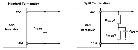
Figure 38. CAN Bus Termination Concepts
