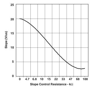
Figure 33. HVD233 Driver Output Signal Slope vs Slope Control Resistance Value
