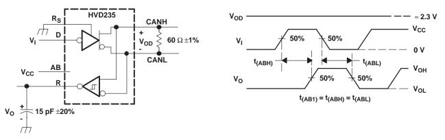
NOTE: All V<sub>1</sub> input pulses are supplied by a generator having the following characteristics:  $t_r$  or  $t_f \le 6$  ns, pulse repetition rate (PRR) = 125 kHz, 50% duty cycle.
