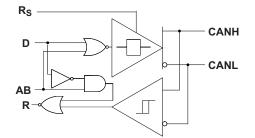
Figure 31. SN65HVD35 Functional Block Diagram
