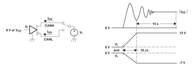
Figure 26. I<sub>OS</sub> Test Circuit and Waveforms
