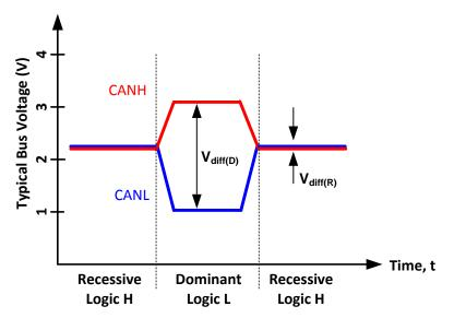
Figure 34. Bus States (Physical Bit Representation)
