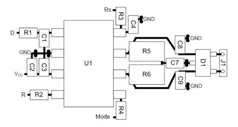
Figure 41. Layout Example Schematic
