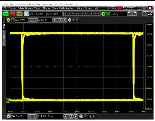
Figure 9-6. Eye Diagram at 4 Mbps PRBS 2<sup>16</sup> – 1, 5 V and 25°C
