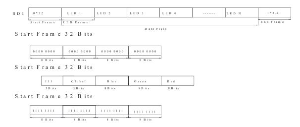
Product structure: GRB order output light, optimize the product blending effect (adjusted IC default RGB order wafer position)
