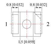
**Recommended Soldering Pad Dimensions**
