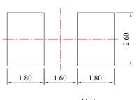
Unit: mm Tolerance: ± 0.10mm
