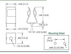
\*Fuse clips without end stops are not UL recognized
