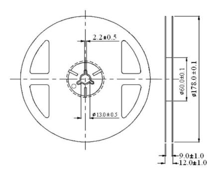
Unit: mm Tolerance:  $\pm 0.25$ mm
