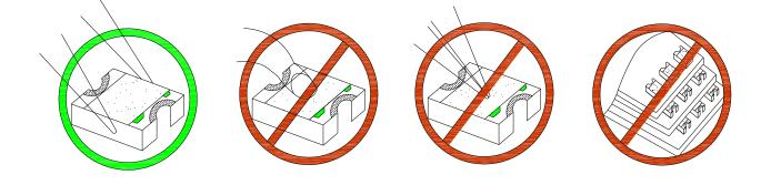
Compare to epoxy encapsulant that is hard and brittle, silicone is softer and flexible. Although its characteristic significantly reduces thermal stress, it is more susceptible to damage by external mechanical force. As a result, special handling precautions need to be observed during assembly using silicone encapsulated LED products. Failure to comply might lead to damage and premature failure of the LED.
