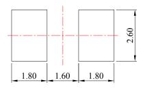
Unit: mm Tolerance: ± 0.10mm
