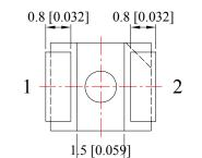
**Recommended Soldering Pad Dimensions**
